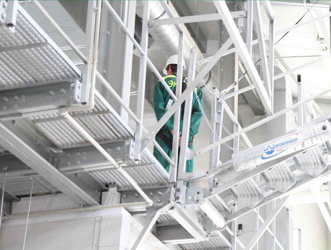
Hydraulic folding ladder located on the bridge that ensures safety when conducting work on a tank-container
