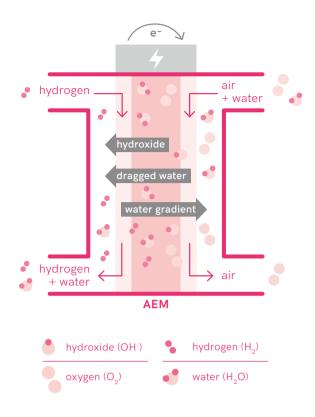
Source: Dekel, D. (2018) Review of cell performance in anion exchange membrane fuel cells
